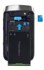
To remove the media card, press the media card in and then pull it out.
